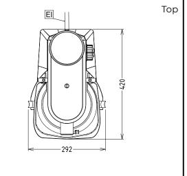
Electric Supply voltage: 600140 (DBE8BYA) 200-240 V/1N ph/50/60 Hz **Electrical power max.:** 0.6 kW **Total Watts:** 0.6 kW Capacity: Performance (up to): 2.5 kg/Cycle **Capacity:** 8 litres Key Information: **External dimensions,** 292 mm Width: **External dimensions,** Depth: 416 mm External dimensions, Height: 527 mm Shipping weight: ISO 9001; ISO 14001 kg Net weight (kg): 19 Cold water paste: 2.5 kg with Spiral hook Egg whites: 14 with Whisk
